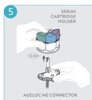
**Insert the top of the Device Connector** (white side) into the **bottom** of the **Serum Cartridge Holder** (also white) until it clicks.
