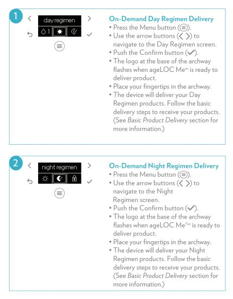
NOTE: The device will deliver the product according to the delivery method you have selected. If you are using the Semi-Automatic delivery method, you will need to push the Confirm button for the device to deliver your product. If you are using the Automatic delivery method, the device will automatically deliver the product when you put your fingertips in the archway.
