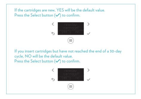
After you insert new cartridges, the device will prime your products. You will hear the device pump a few times before it dispenses each product. Make sure to keep your fingertips in the archway during the whole priming process. The device will deliver the product you primed onto your fingertips.
