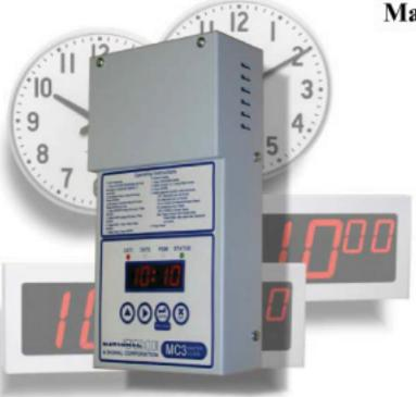
The MC3 Master Clock combined with National's clocks creates a state-of-the-art time system. The MC3 comes standard with three solid state 120VAC outputs to directly control clock circuits without the need for additional relays. These solid state outputs are capable of driving 3 amps each and incorporate zero-cross technology to handle undesirable current surges and inrush.
