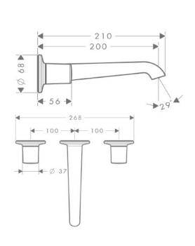
•**Description:** Hansgrohe Axor Bouroullec Three-Hole basin mixer for concealed installation with short spout
