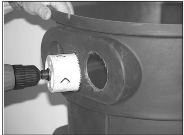
Section 2 - Installation of 2" Bulkhead Fitting in 3" hole
