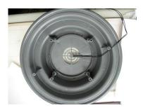
3. Install the motor in vacuum casing and be sure the motor position is same as figure.
