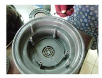
2. Put the gasket into the chamber of vacuum casing (Black or light yellow color).
