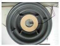
4. Thread the motor cable and magnetic switch cable through the middle casing.
