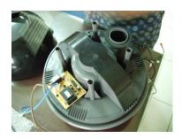
10. After take out the motor, gasket and magnetic switch.
