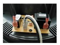
7. Connect the magnetic switch cable with printed circuit board terminal.
