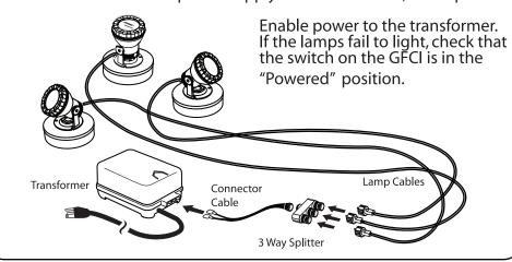
**NOTE:** It is important for the transformer to be protected from weather by a cover. All outdoor receptacles, especially ground fault circuit interrupter (GFCI) types should be protected. Some ideas for this are:
