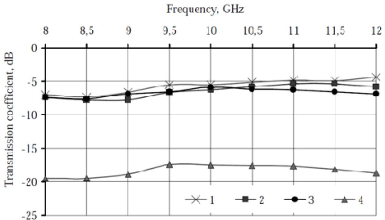
Figure 2. Frequency dependence of the transmission coefficient for shungite annealed in the oxidizing conditions (1); in a chamber with  $\text{NH}_4\text{Cl}$  (2); in vacuum (3); and for unannealing shungite (4).
