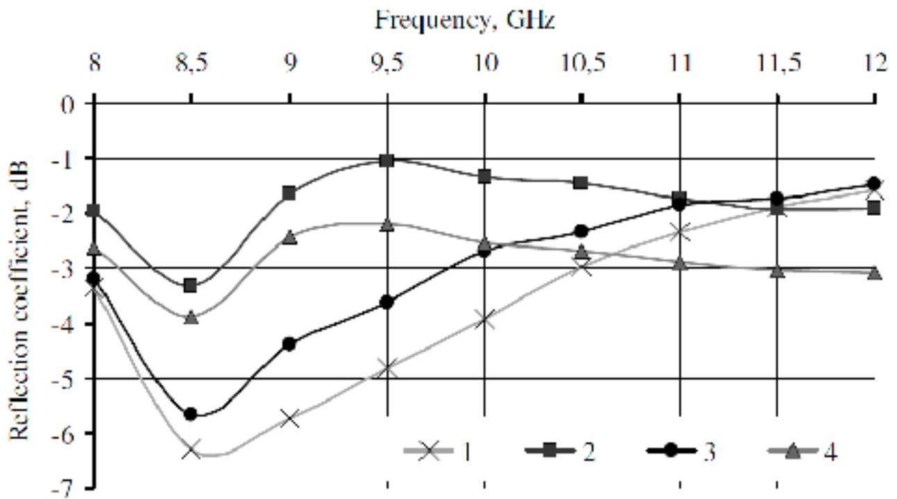
Figure 3. Frequency dependence of the reflection coefficient with metal reflector for shungite annealed in the oxidizing conditions (1); in a chamber with  $\text{NH}_4\text{Cl}$  (2); in vacuum (3); and for unannealing shungite (4).
