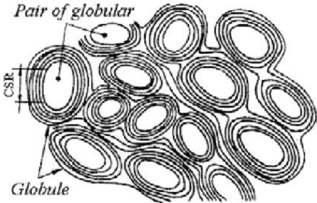
*Figure 1. Model of a globular structure of shungite carbon [4].*
