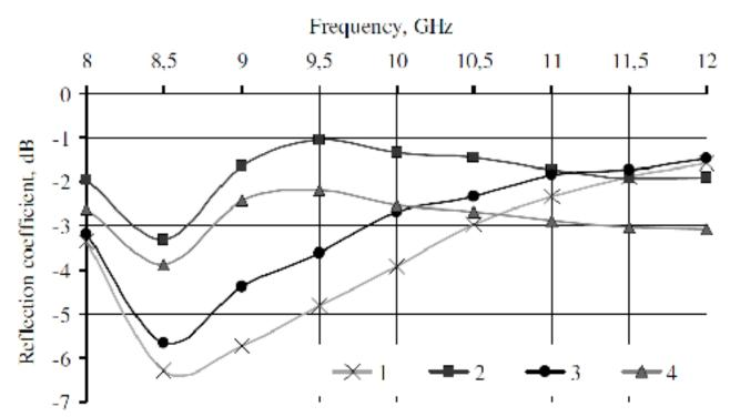
Figure 3. Frequency dependence of the reflection coefficient with metal reflector for shungite annealed in the oxidizing conditions (1); in a chamber with NH4Cl (2); in vacuum (3); and for unannealing shungite (4).
