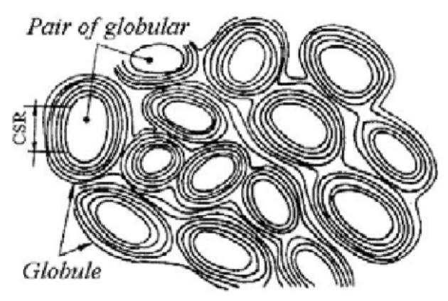
Figure 1. Model of a globular structure of shungite carbon [4].
