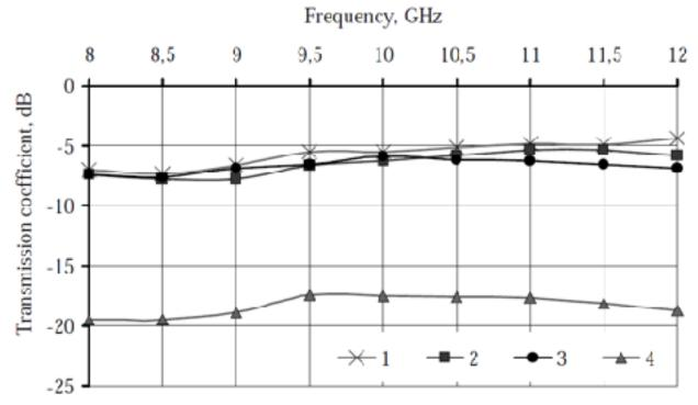
Figure 2. Frequency dependence of the transmission coefficient for shungite annealed in the oxidizing conditions (1); in a chamber with NH4Cl (2); in vacuum (3); and for unannealing shungite (4).
