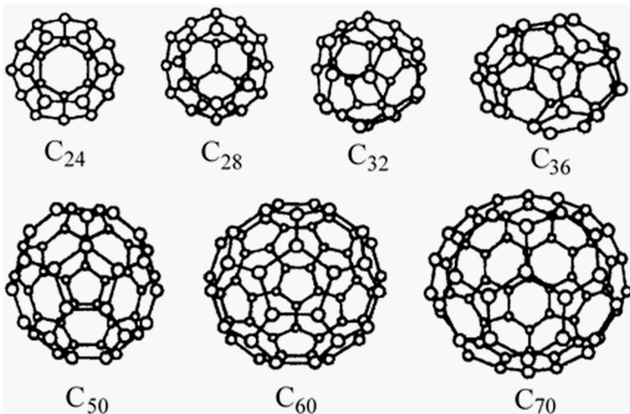
Figure 4: Varieties of natural and synthetic fullerenes with different numbers of carbon atoms:  $C_{24}$ ,  $C_{28}$ ,  $C_{32}$ ,  $C_{36}$ ,  $C_{50}$ ,  $C_{60}$ ,  $C_{70}$ .
