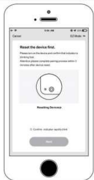
6. Confirm indicator rapidly blink, press Next button.
