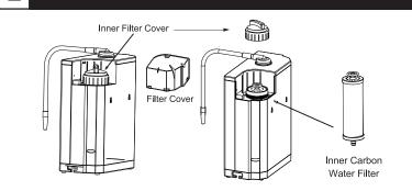
Remove the outer filter cover by pressing on top and pulling up. Twist the inner filter cover counter-clockwise to open. Prime a new inner filter by holding it under running water for 3-5 minutes with the water going into the side with the 2 black o-rings. Insert the inner carbon filter into the filter chamber and press firmly. Replace the inner filter cover and the filter cover.
