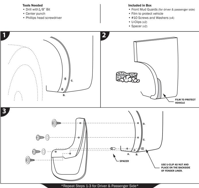
**STEP 1.** Remove existing fasteners.
