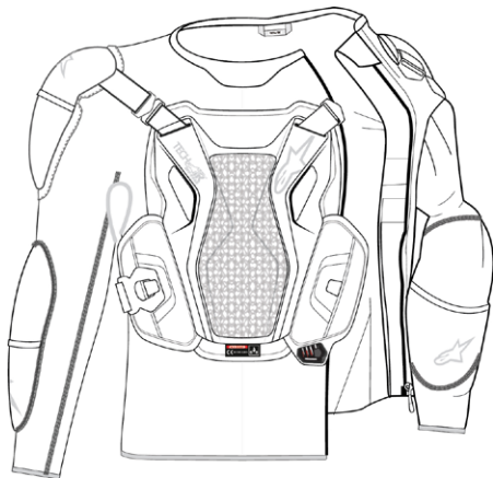
Figure 14: System switch off via opening of Activation Zip (1)
