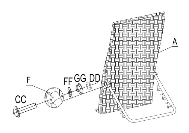
Connect A and B with CC&FF&GG&DD, two sides together. If will be used this step.
