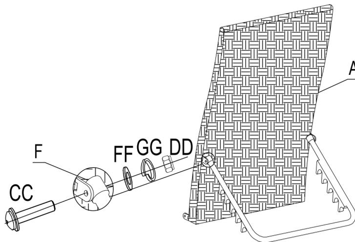
Connect A and B with CC&FF&GG&DD,two sides together.
