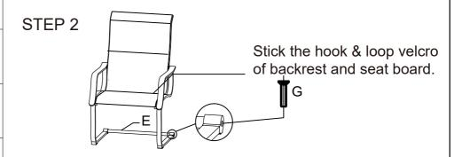
Connect chair leg support beam (E) with legs. M6\*25 (G) are used. Make sure all bolts are inserted properly, then tighten all bolts to the end.
