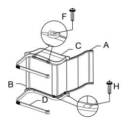
Connect chair back (A) with seat base (B) and armrests (C and D). M6\*20 bolts (F) and M6\*30 bolts (H) are used. Please do not tighten bolts to the end at this step.
