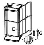
Place chair support beam (E) in the between of chair armrests properly and screw it. M6\*15 bolts (G) are used. Please do not tighten any screws to the end at this step.
