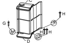
Screw chair armrest (C and D) to chair back (A) and seat board (B). M6\*15 bolts (G) and M6\*30 (H) are used. Please do not tighten screws to the end at this step.
