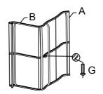
Screw chair back (A) to seat board (B). M6\*15 bolts (G) are used. Please tight screws to the end.
