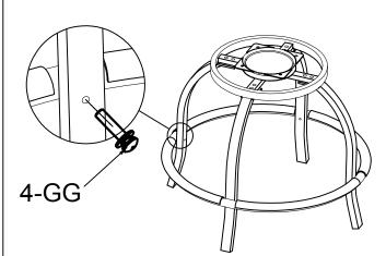
After the completion of Step 2, go back to Step 1 and tighten all the bolts.
