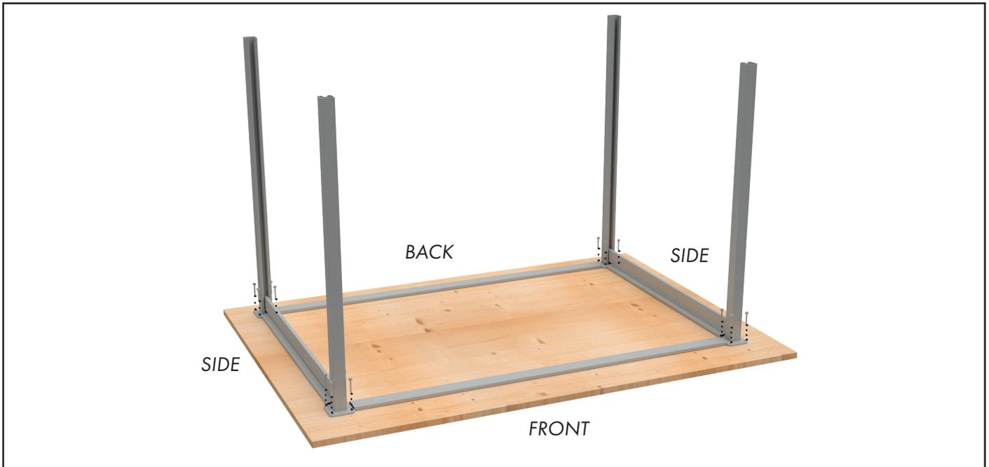
**A** On top of a sacrificial board made from minimum 15mm thick structural timber, position posts using the provided guide slats to measure their location. Check measure the squareness of your layout as well as the outside distance between posts (which should match the defined width and depth of your enclosure). Adjust as necessary before screwing down posts into the sacrificial board.
