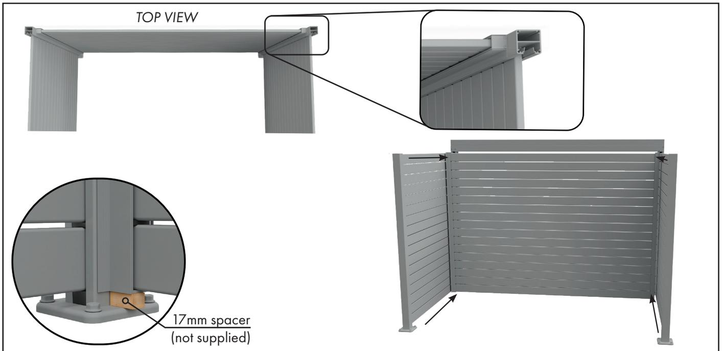
9 Lift back slat assembly into position between back two posts.
