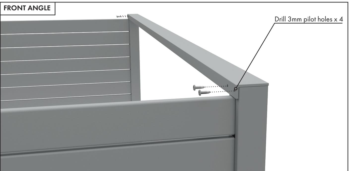
**11 NOTE:** Assembly is shown with closed back from this stage, same steps apply to open back version.
