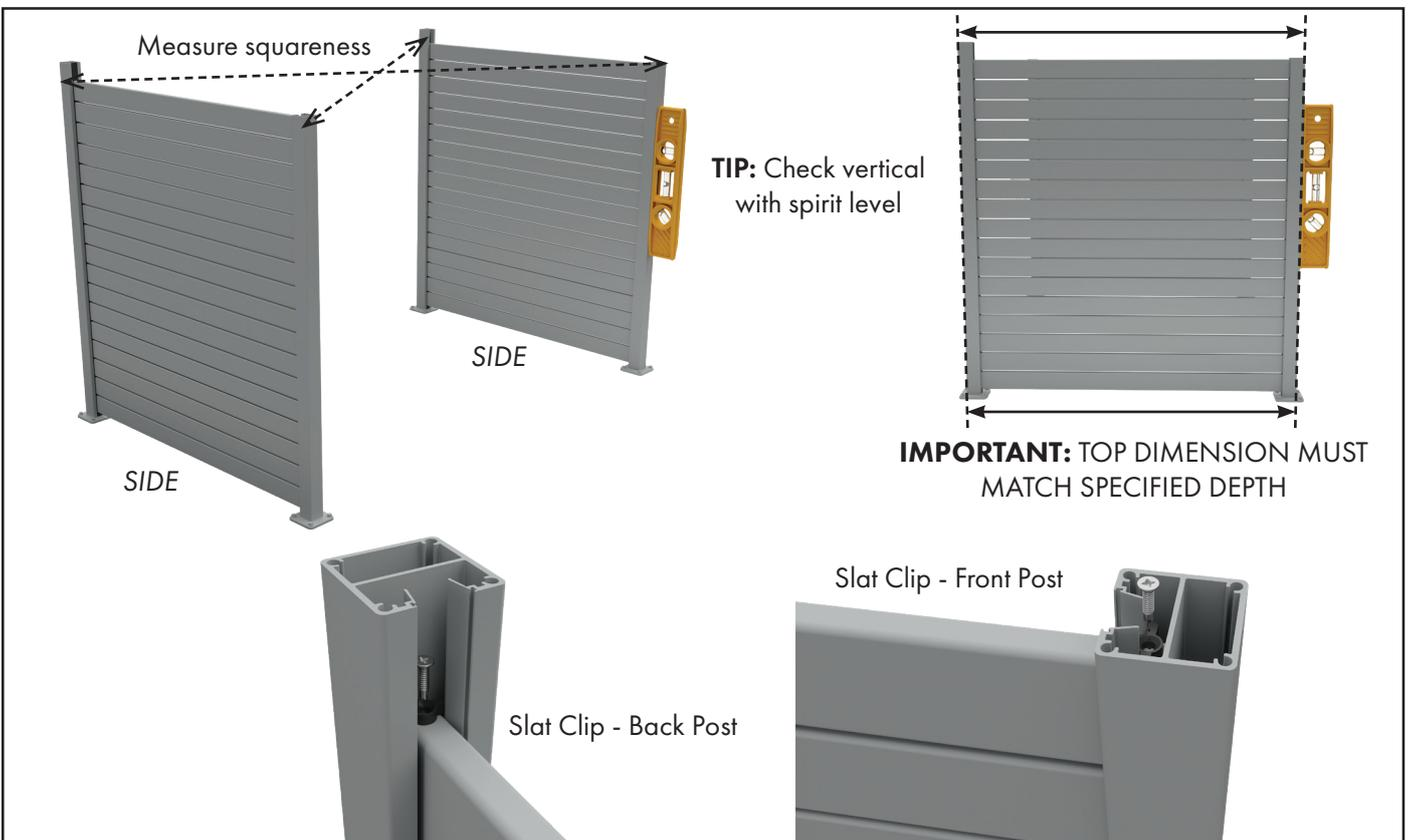
4 Once all slats are in position, check measure squareness of structure at bottom and top on both diagonals. **IMPORTANT:** Measure the depth of your structure from top of outside edge of side posts (see above). This must match the depth of your enclosure (and also match the depth of the structure at the bottom of posts). If posts are not positioned correctly, the lid will not fit. Adjust as necessary using a padded mallet to move the post inwards or outwards.
