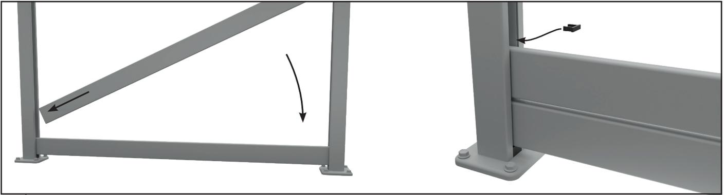
3 Build the enclosure SIDES by pivoting slats into position. Insert a spacer block above the first slat, followed by a slat, inserting into one post and levering the other side into the other post. Alternate between spacer blocks and slats. Do not install a spacer block on top of the final top slats. Use a rubber mallet if needed to ensure slats are fully pushed down in post.
