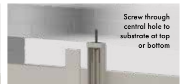
Screw top/bottom plate to centre support rail
