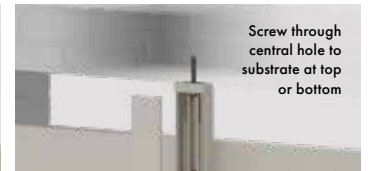
Screw top/bottom plate to centre support rail
