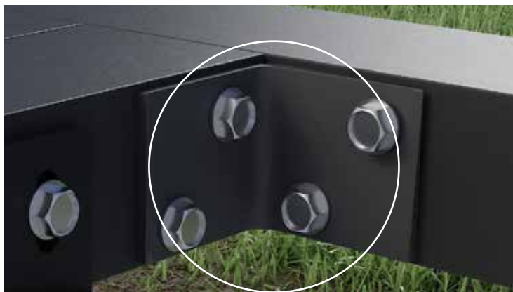
'Picture frame' ends if subframe not constrained between walls. Butt aluminium 55x40x3mm joist to ends of adjacent aluminium joists and secure in place with 40mm high angle
