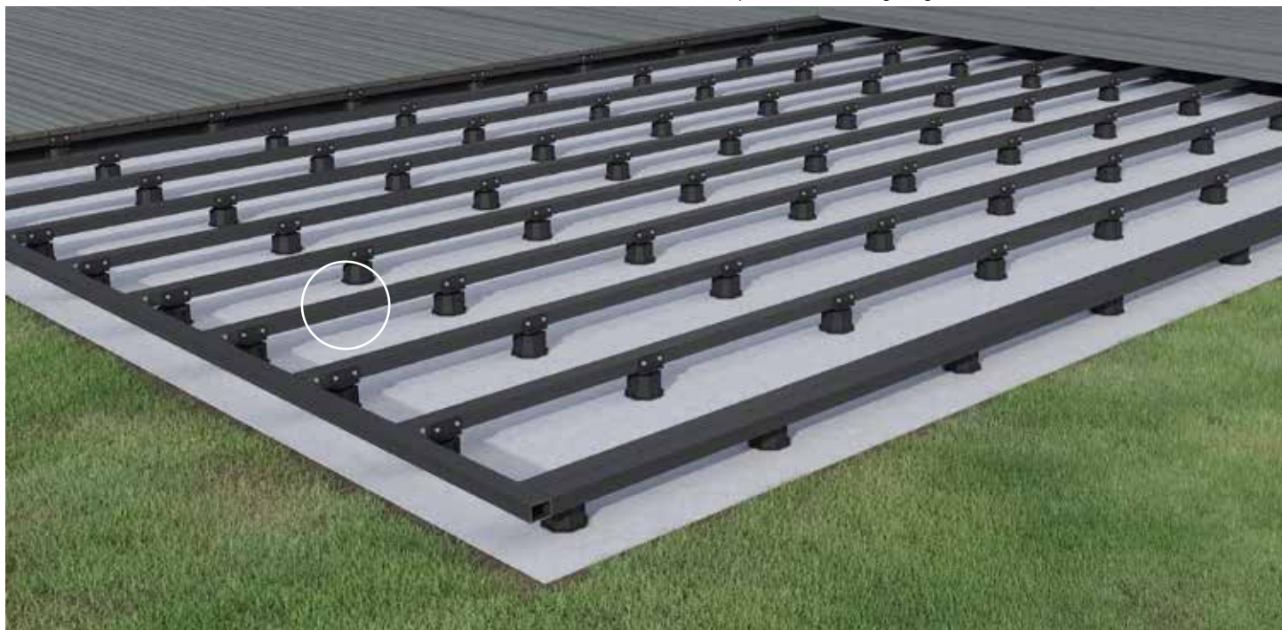
'Picture frame' ends if subframe not constrained between walls. Butt aluminium 55x40x3mm joist to ends of adjacent aluminium joists and secure in place with 40mm high angle
