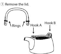
② Pull up the rings and insert "Hook A." Gently open up "Hook B."
