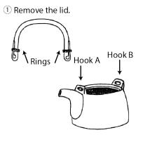
② Pull up the rings and insert "Hook A." Gently open up "Hook B."
