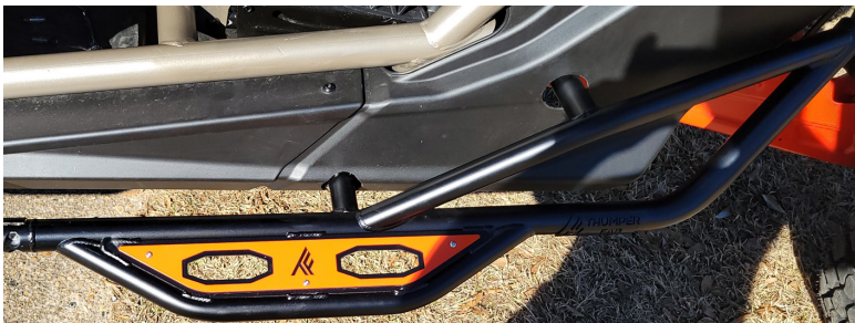
FIG 6 - Install Rear Nerf Rail
