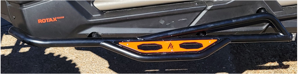
FIG 4 - Install Front Nerf Rail
