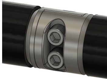
FIG 7 - Fasten Bungs Together (1/4" Allen Wrench)
