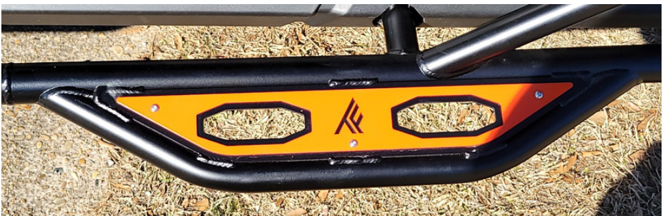
FIG 8 - Install Accent Panels (3/32" Allen Wrench)
