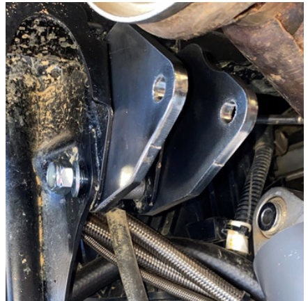
(FIG 9) Install REAR - Outer Lift Bracket using 15mm Socket and 15mm Wrench
