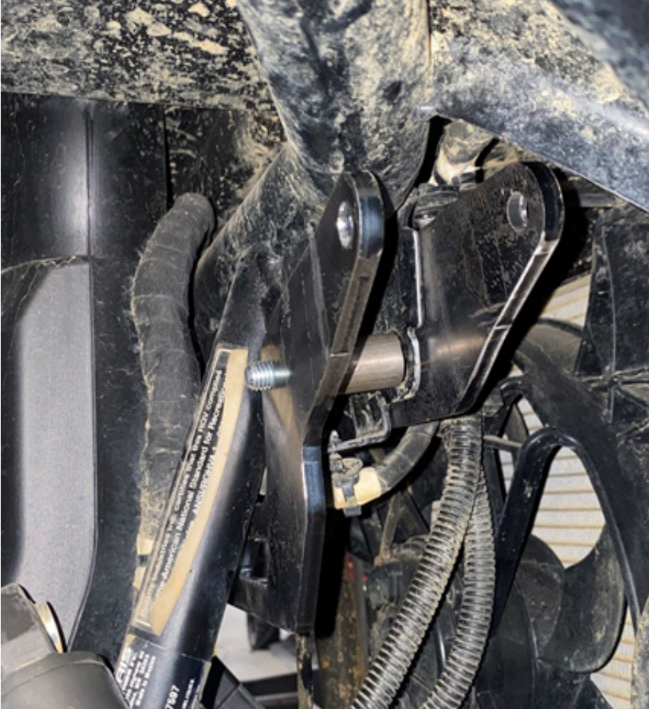
FIG 2 - Install FRONT - Inner and Outer Lift Brackets using 15mm Socket and 15mm Wrench
