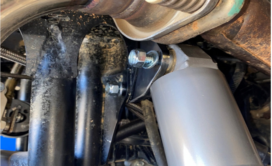
FIG 10 - Tighten REAR - Inner and Outer Lift Brackets (3&4) into place using 15mm Socket and 15mm Wrench
