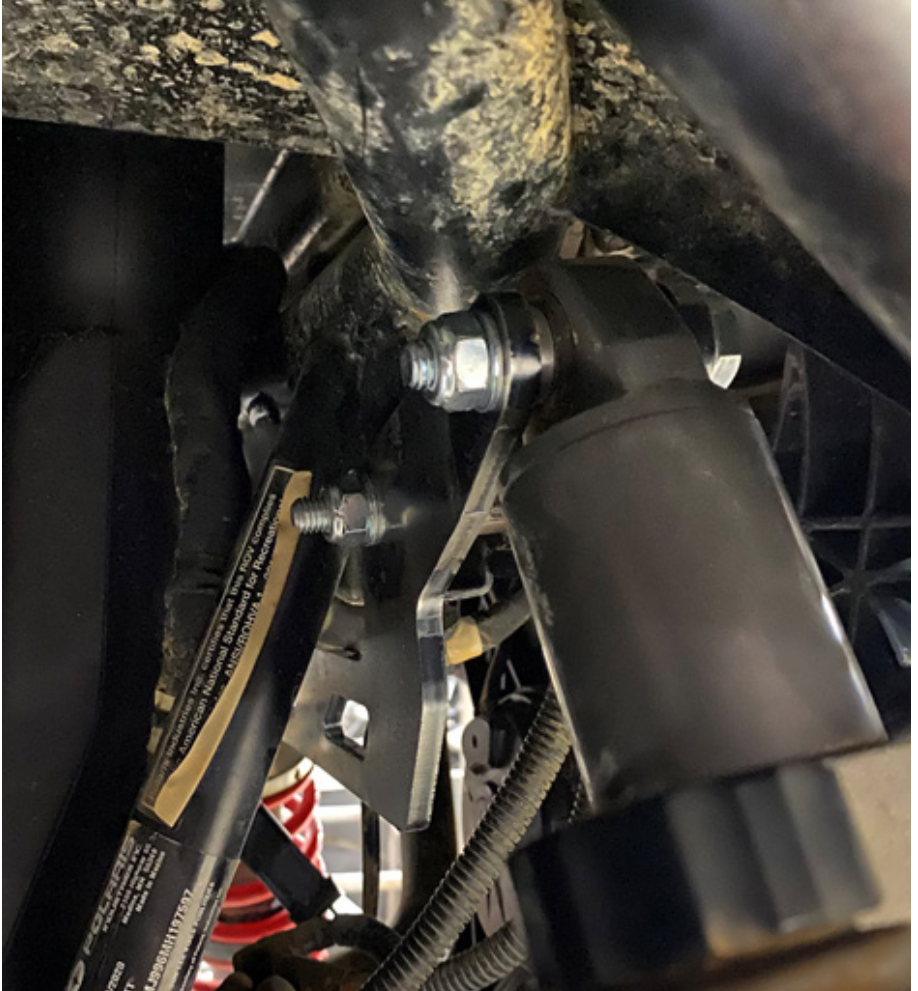
FIG 3 - Reinstall shock and tighten Flange Bolts (A&B) using 15mm Socket and 15mm Wrench
