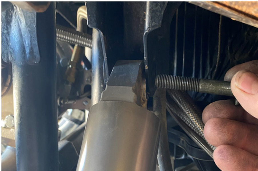
FIG 6 - Remove the Upper Shock Mounting Bolt using 15mm Wrench and 15mm Socket
