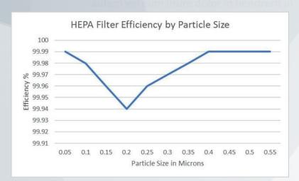
The chart represents the efficiency of HEPA filters in relation to the filtered particle size. As the particle size goes down, the filter will be less likely to intercept them directly, but at the same time, their random movement makes them more likely to encounter the filtering fibers. As the particles increase in size, the particles will be easily intercepted by the fibers (4).
