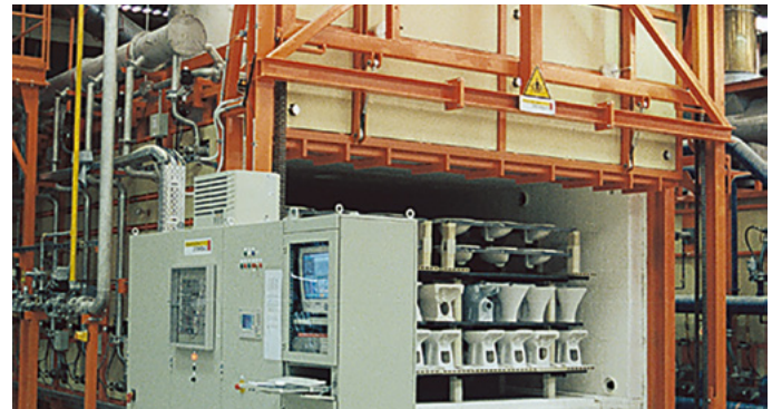
Intermittent shuttle kiln in the ceramics industry
