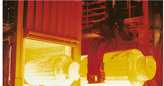
Bogie hearth forging furnace in the metallurgical industry
