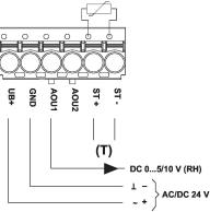
Connectors ST+ / ST- are only used for sensor types which additionally have a passive resistance sensor element for temperature measurement.
