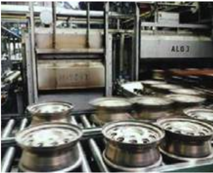
Aluminium industry: curing oven for wheel rims
