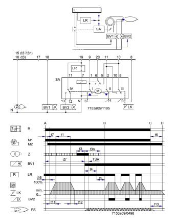
Load control with a 2-position controller. During burner off times, the air damper is closed.
