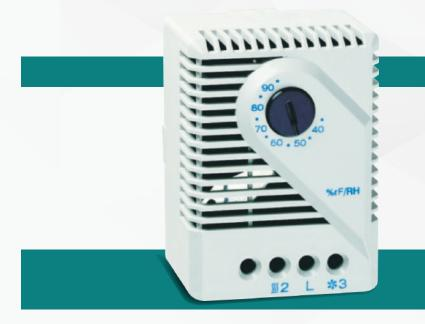
The HS01 is designed to control the relative air humidity inside of enclosures. When connected to an enclosure heater, (de-humidifier), it will turn the heater on at the set humidity level in order to raise the dew point. This helps prevent damage and malfunction of electronic components caused by condensation and corrosion\*. The HS01 can also be used to control cooling fans, warning lights or other devices.
