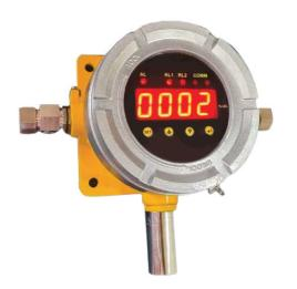
Equipped with a Japanese catalytic combustion sensor, the instrument ensures reliable measurement of Hydrogen, Methane, Isobutane, Propane, and LPG. Featuring a 0-100% measuring range, a 4-20mA output, and optional relay and RS-485 Modbus communication, the GS-LEL-01 offers flexibility and adaptability to diverse operational needs.
