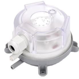
The DPS01 is an adjustable differential pressure switch capable of detecting minuscule changes in pressure. The switch set point can be field-adjusted without the need of a manometer by using the adjustment knob and the built-in calibrated visual scale. This switch is equipped with a clear cover that protects the adjustment knob from involuntary movement and also provides class IP54 protection.
