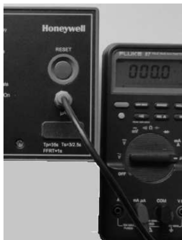
Fig. 4-3: Measuring flame signal with multi meter ( \mu\text{A} range selection) using a jack plug.
