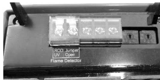
ULT Model (bus connector and address switches)
