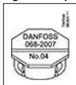
Figure 7: Capillary tube label for T2 and TE2
