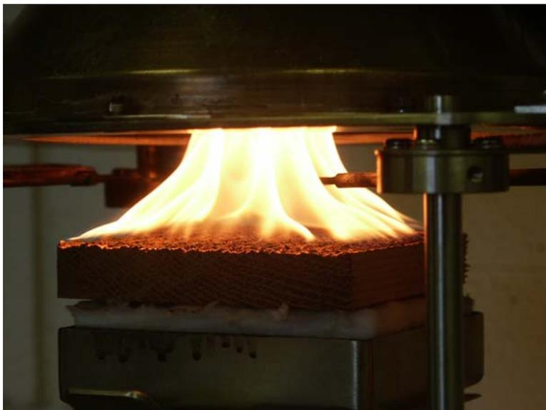
c) Sample after 30+ seconds, flaming initiated using spark pilot
