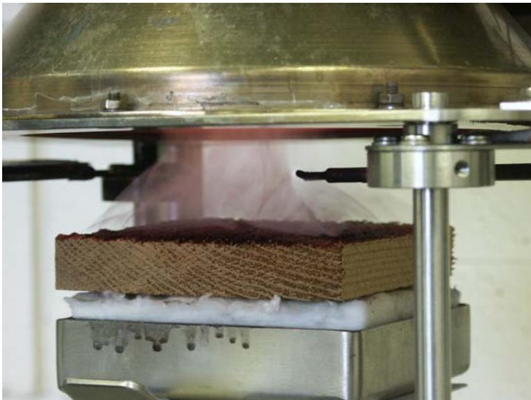
b) Sample exposed for 20 seconds, decomposition products almost in quantities sufficient for combustion
