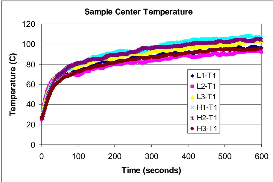
Figure 8 Summary Plot of Measured Center Temperature, Light and Heavy Weight Materials.
