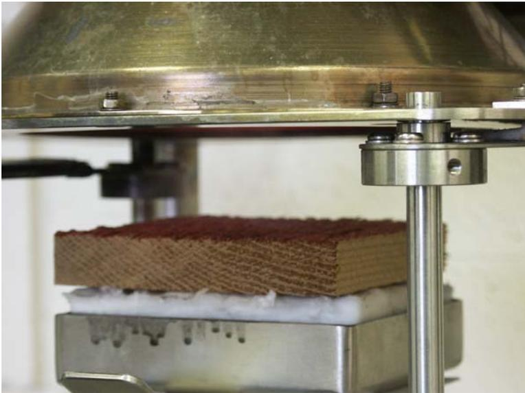
a) Sample exposed for approximately 10 seconds - starting to smoke
