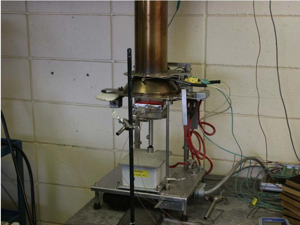
**Figure 2 Cone Calorimeter Used for Evaluation of Firezat Samples**
