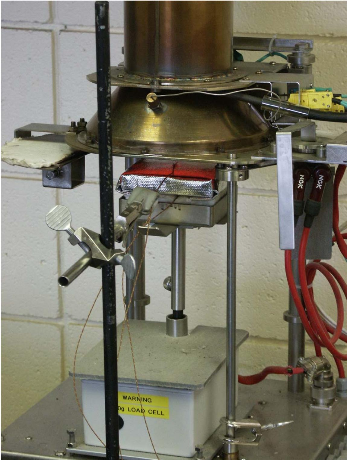
Figure 5 Sample Under Cone Calorimeter During Exposure
