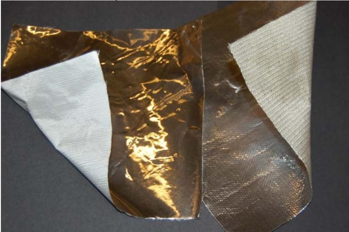
**Figure 1 Fire Barrier Materials Evaluated Using Cone Calorimeter (light weight, heavy weight)**
