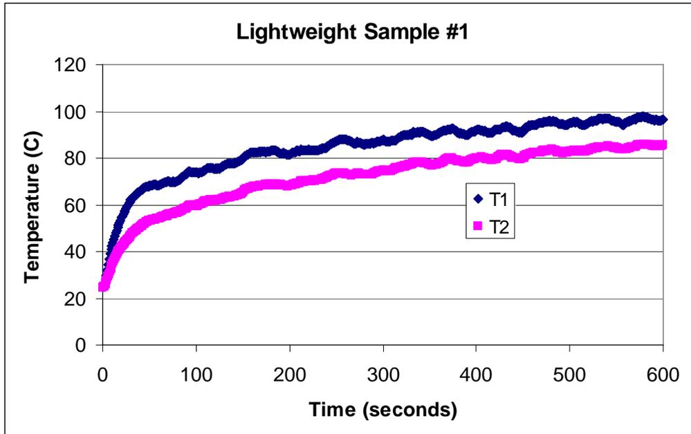
Figure 6 Lightweight Material Exposed at  $33 \text{ kW/m}^2$  for 10 minutes
