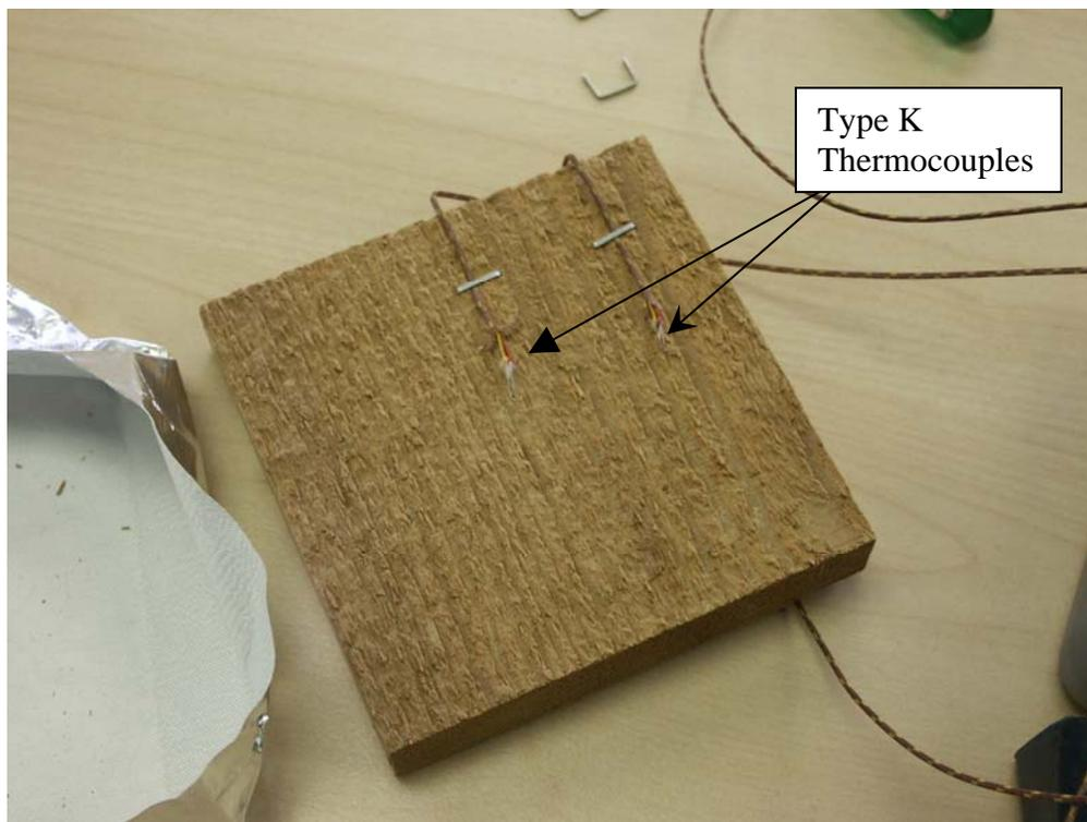
**Figure 4 Sample of Cedar Wrapped Prior to Wrapping in Firezat Material**
