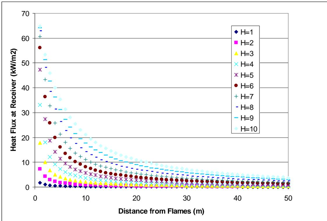
Figure 3 Simulated Heat Flux from a Planar Flame at a Distance from a Receiving Surface
