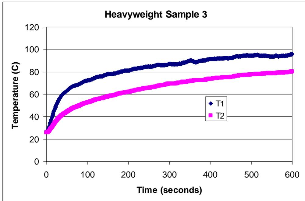
**Figure 7 Response of Heavy Weight Barrier Material to Heat Flux of 33 kW/m<sup>2</sup>.**
