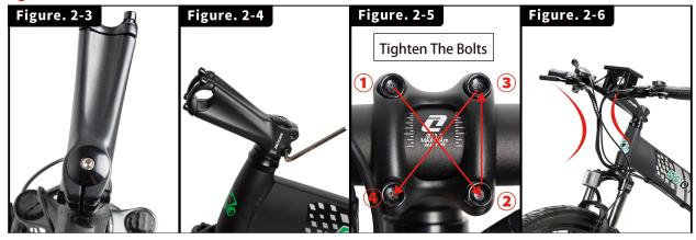
4. Unscrew the two screws on display, then install the display on the center of the handlebar(the rubber gasket is necessary for this bike), then install the control panel (the buttons) on the driver side of the handle, then connect the quick release connector, it has arrows on both ends of the connector, you can plug the connector easily with aligning arrows (Figure 2-6). Unscrew the bolt on the front of the fork, then install the front reflector.
