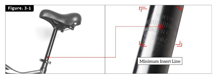
2. Open the clamp on the seat tube, insert the seat post into the seat tube, adjust the seat to a comfortable height, tighten the tension adjusting nut, and press the clamp lever inward toward the seat tube (Figure. 3-2).
