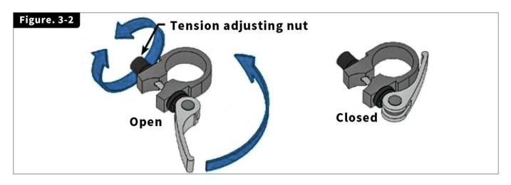
**Please Note**: If necessary, tighten the clamp by twisting the clamp handle clockwise while in the un-clamped position. Then, fold the handle in toward the seat post. This should require a fair amount of force to ensure the seat post is held tight. If necessary, the clamp can be further tightened with a 5 mm Allen wrench while in the clamped position.
