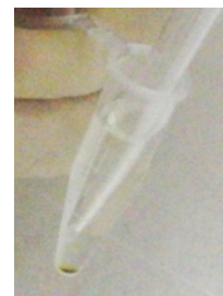
Figure 7: A pipette is inserted 1-2 mm from the nanoparticle pellet as the supernatant is gently removed.
