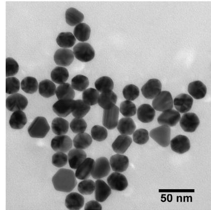
Figure 3: TEM image of a NIST gold nanoparticle reference material (RM8012) used for intermediate magnification calibration.
