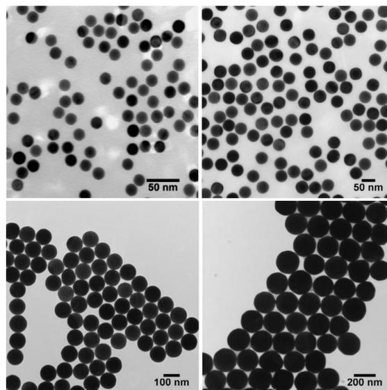
Figure 1: Transmission electron microscope (TEM) images of ultra uniform gold nanoparticles between 20 nm and 200 nm in diameter.
