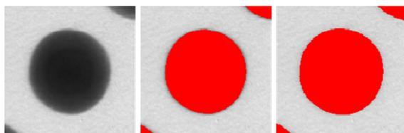
Figure 8: A magnified TEM image of a single particle (left). Applying the default threshold settings (center) in ImageJ produces a red selection with a dark ring, the latter corresponding to lower-contrast edge pixels. Adjusting the threshold values to increase the range of grey values selected (right) accurately selects the edge pixels for sizing.
