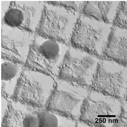
Figure 2: TEM image a grating replica with deposited latex spheres for low magnification calibration.
