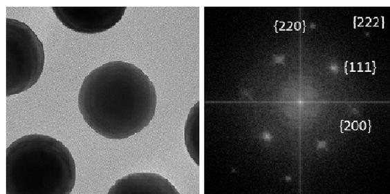
Figure 6: High-resolution TEM image (left) of ultra uniform gold nanoparticles. The calculated FFT (right) of the central particle shows diffraction spots from the gold lattice along the [011] zone axis.
