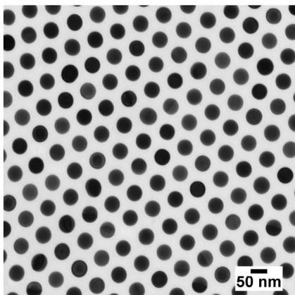
Figure 5: TEM image of polymer-coated ultra uniform gold nanoparticles.
