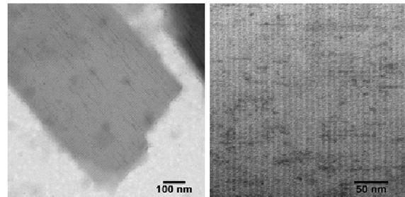
Figure 4: TEM image of a beef catalase crystal used for high magnification calibration at low magnification (left) to show the crystal morphology and at higher magnification (right) to illustrate the internal lattice structure of the crystal.
