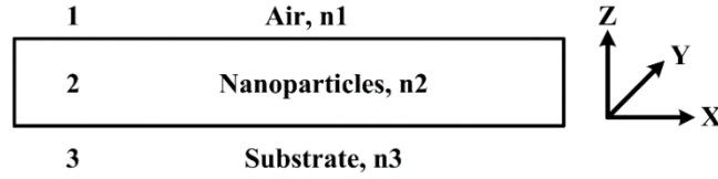
Figure S10. The geometry of three-layer structure
