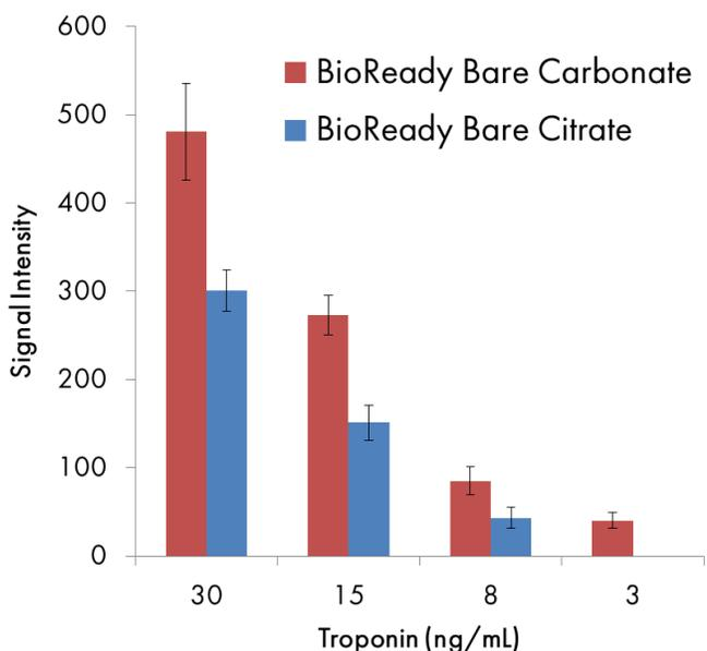
**Figure 6.** Signal intensity of test line in lateral flow strips using anti-cTnI conjugates on either carbonate buffered BioReady Bare particles or Citrate buffered BioReady Bare particles.
