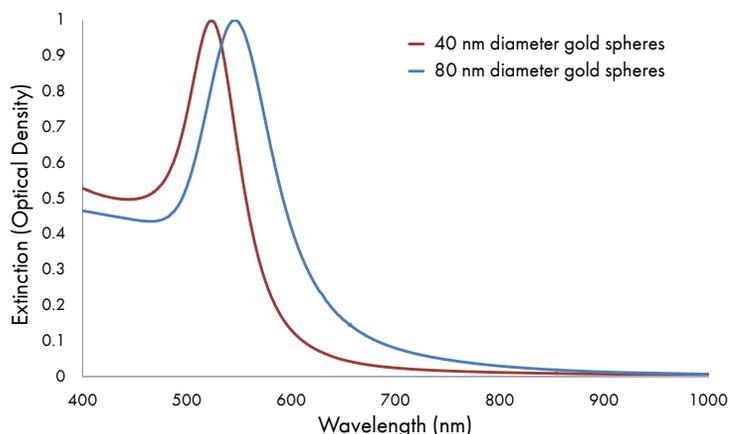
**Figure 4.** UV-Visible spectra of 1 OD 40 nm and 1 OD 80 nm gold nanoparticles.
