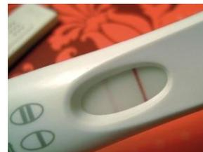
**Figure 1.** The commercial pregnancy test uses gold nanoparticles for detection. The faint red line indicates a positive result. The dark red line is the control.
