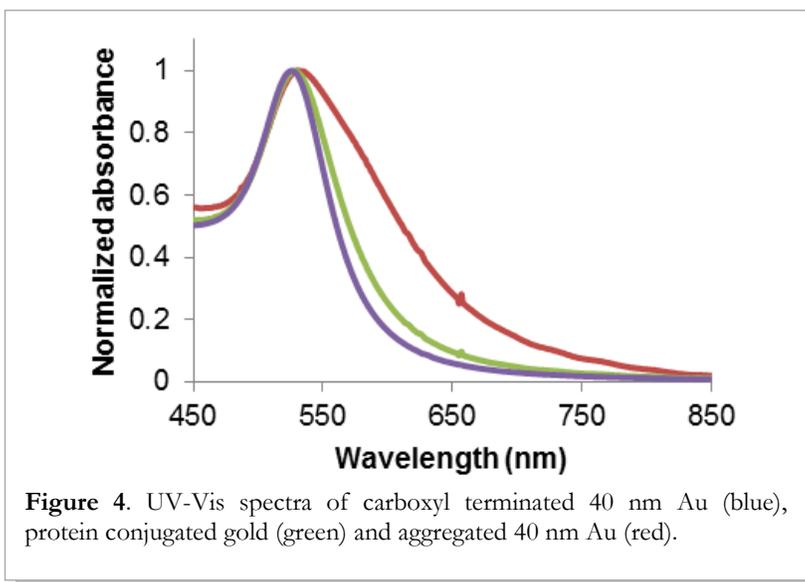
**Figure 4.** UV-Vis spectra of carboxyl terminated 40 nm Au (blue), protein conjugated gold (green) and aggregated 40 nm Au (red).
