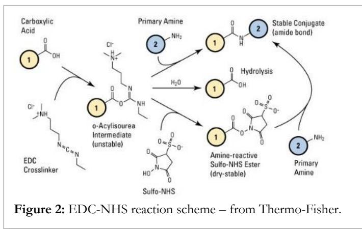
**Figure 2:** EDC-NHS reaction scheme – from Thermo-Fisher.
