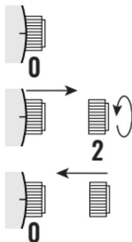
\* Do not set the date between 9:00 P.M. and 3:00 A.M. , otherwise the day may not change properly. If it is necessary to set the date during the time period, first change the time to any time outside it, set the date and then reset the correct time. 5
