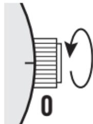
**TO UNSCREW:** Turn the crown anti-clockwise until it turns freely without tension. GENTLY pull the crown out to the other desired positions for watch setting (see specific operating instructions on the following pages).
