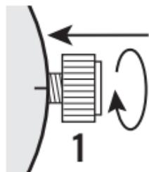
**TO SCREW:** Push the crown ALL THE WAY IN (towards the watch) THEN begin to turn clockwise until it is securely screwed down.
