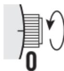
1. Unscrew the crown by turning it anti-clockwise.
