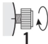
2. When it is in position [1], turn the crown clockwise to wind. Wind 5-10 times and it will start to move naturally after shaking slightly.
