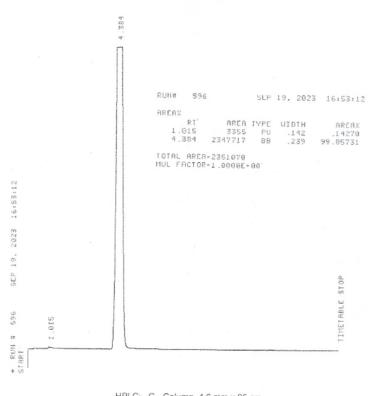
$\begin{array}{c} \text{HPLC: } \quad \text{C}_{\text{18}} \text{ Column, 4.6 mm x 25 cm} \\ \text{Acetonitrile/Methanol/Water} \quad 37/37/26 \\ \quad 2 \quad \text{mL/min} \\ \quad \text{UV}_{\text{254}} \text{ Detection} \end{array}$
