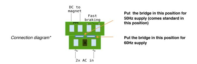
\*The VIS standard series is supplied with a special rectifier suitable for AC 220 to 500 with fixed DC output. Move the frequency bridge in the right position before connecting the brake. Rectifiers come from factory with ridge connected for 50Hz supply.
