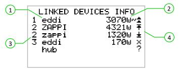
This screen lists all the linked devices 1 and the priority setting for each device 3 The current device is shown in CAPITAL letters. To the right of each device is the real-time output power level 2 The right side of the screen has symbols to show the status of each device 4 Refer to the table on the next page for the meaning of each symbol.
