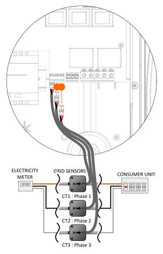
**SINGLE PHASE:** A CT clamp must be placed around the live meter tail as shown above with the arrow pointing towards the consumer unit.
