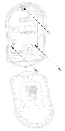
Using the fixing kit provided secure unit to the wall ensuring the grommets are used to maintain its IP integrity (Note: if using the rear cable entry remember to insert the mains cable before mounting to the wall!)
