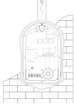
Using zoppi template mark mounting holes. Use top and 2 bottom holes left/right for brick use 2 vertical holes if mounting to a stud wall or joist. 6
