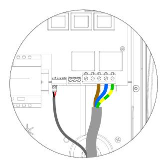
For single phase installations where 1 or 2 external / additional CT's are required, please follow the above diagram to connect the CT's using the extra 2 CT terminals in the same way if required.
