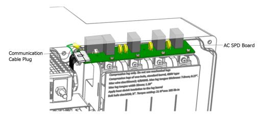
Figure 1: Disconnecting the Plug of the Communication Cable of AC SPD Board
