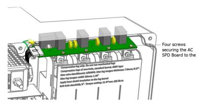
Figure 2: Disconnecting the AC SPD Board From the AC Conductors
