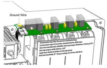
Figure 3: AC SPD Board Removal
