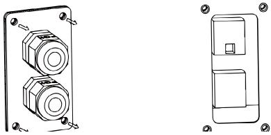
Step 2: Prepare a standard network cable and cable connector, then insert the network cable through the cable connector.
