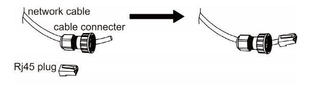
Step 4: Insert the cable connector into COM port at the bottom of energy station and screw it tightly. Then insert other side of the network cable into PC or other device.
